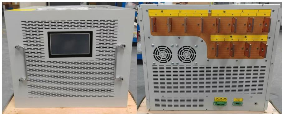
SW-STS, allows instantaneous transfer of power sources to the load. If one power source fails, the STS switches to the back-up power source so fast that the load never recognises the transfer made.
